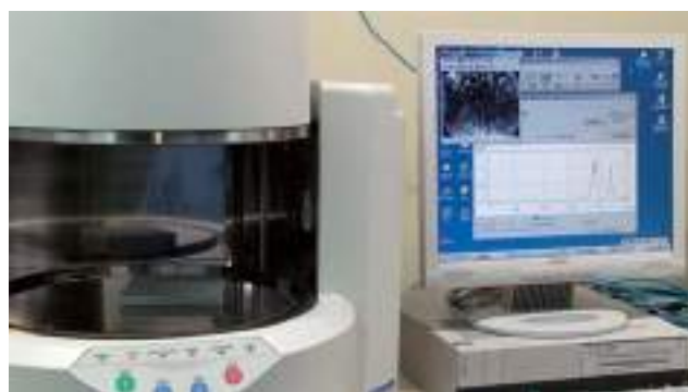
X-ray fluorescence analyzer (RoHS analyzer)
